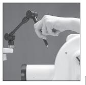
Position of fixation lamp for photogra phing the posterior pole
