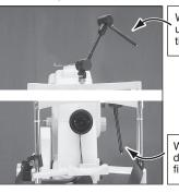
When photographing upward, direct the fixation lamp upward.
