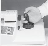
Automatic insertion of exciter filter.
