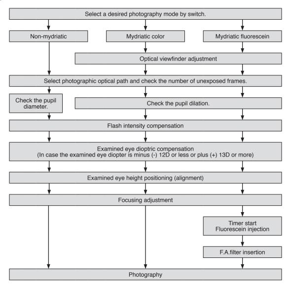
Photography by this instrument is classified into non-mydriatic/mydriatic color, mydriatic fluorescein photography. It is recommendable to grasp a rough operations' flow along the purpose of each photography. If malfunction should occur on this equipment, an alarm will buzz.
